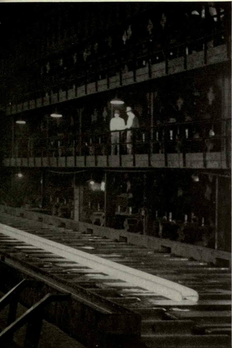
A white-hot steel beam moves along the runway from the final shaping rolls of a U. S. Steel structural mill.
